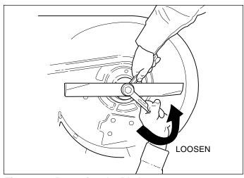
Figure 26. Removing the Blade
